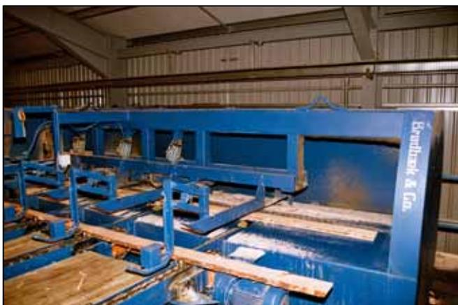
The new BCO 800/60 at work, producing up to 50 boards/min.
